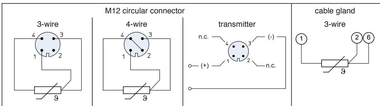
Figure 1: Pin assignment
