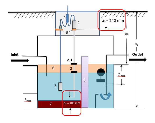
$O_{max}$  = maximum oil layer thickness
