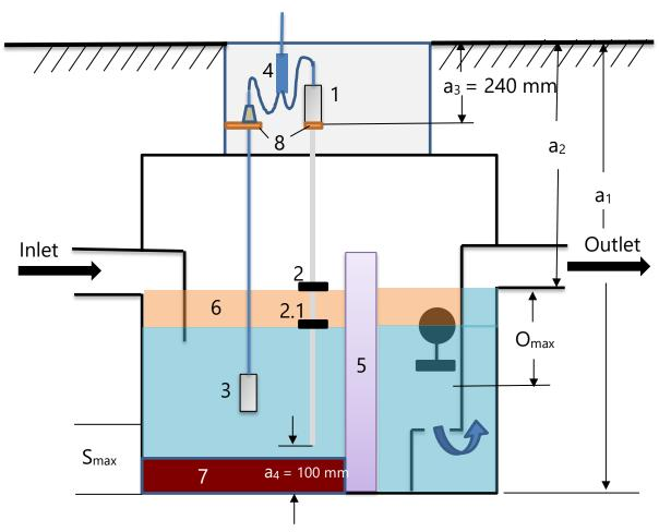
$O_{max}$  = maximum oil layer thickness
