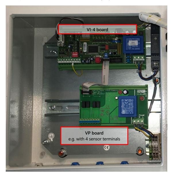
Figure 2: VISY-Command 4 Web, inner view
