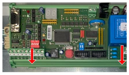
Figure 7: VI-4 Board, fixing
