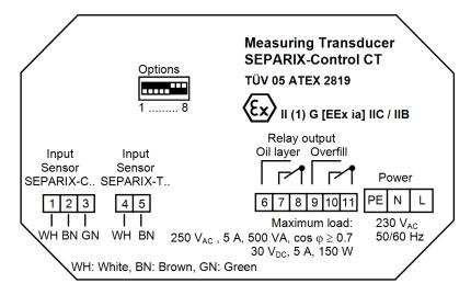
Figure 6: SEPARIX-Control CT, terminals and "Options" DIP switch
