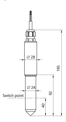
Figure 1: SEPARIX-C L Plus, dimensions
