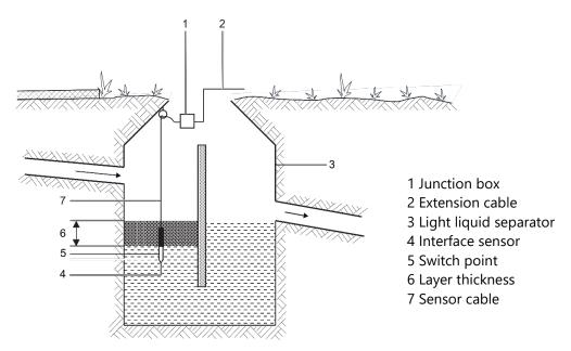
Figure 3: SEPARIX-C, installation
