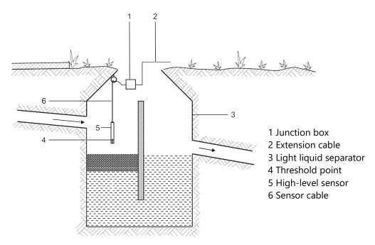
Figure 4: SEPARIX-T, installation
