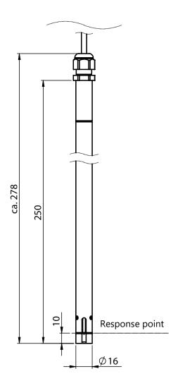
Figure 2: SEPARIX-T L Plus, dimensions
