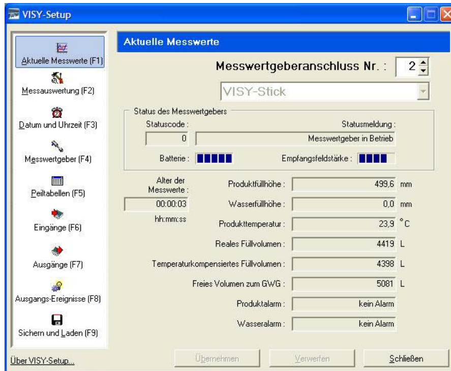
Figure 16: "Current Values" menu in VISY-Setup showing "Age of measured values", "RF Field Strength" and "Battery"
