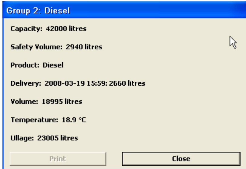
Figure 5: tank group detail display
